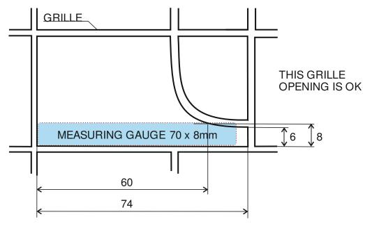
IN THIS EXAMPLE ONE OF THE GRILLE OPENINGS IS MEASURED TO 74mm.
