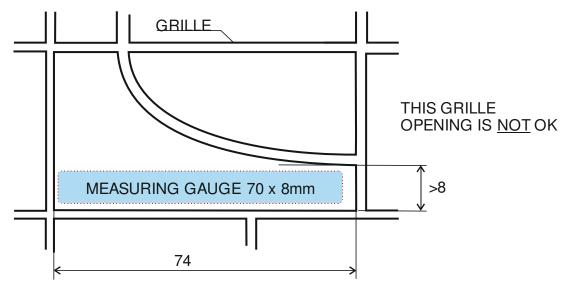
IN THIS EXAMPLE ONE OF THE GRILLE OPENINGS IS MEASURED TO 74mm.
